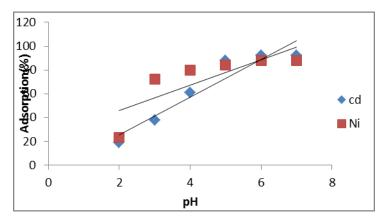
Figure 1: The effect of pH on biosorption of  $Cd^{2+}$  and  $Ni^{2+}$  ions.
