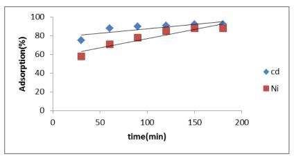
Figure 2: biosorption kinetics of Cd<sup>2+</sup> and Ni<sup>2+</sup> ions.
